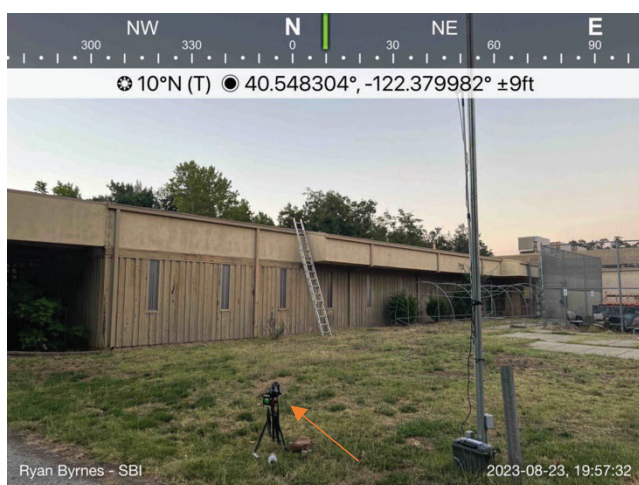
Photo 1. Night vision and bat detector set up on the southwestern side of the Old Juvenile Justice Center during the night emergence surveys. Orange arrow indicating the night vision unit used to monitor for emerging bats.
